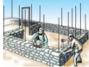
Reinforcement in stone masonry wall
