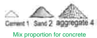
Mix proportion for concrete
